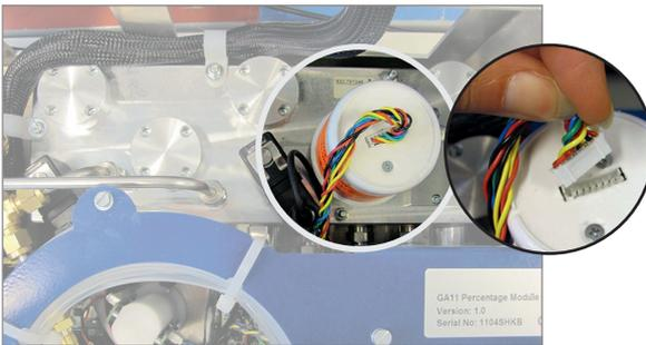
3. Screw out the sensor anticlockwise.
