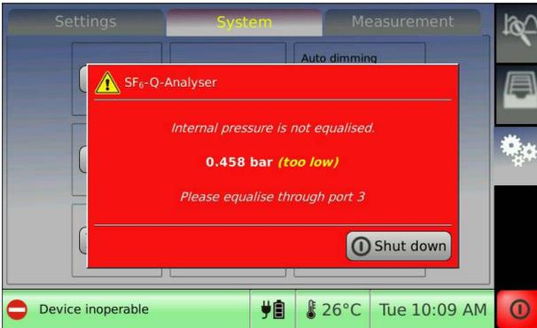
For pressure compensation, connect a gas recovery bag with the desired gas (under atmospheric pressure, max. 1,200 mbar abs. or 200 mbar gauge) to the outlet for the gas recovery bag ③.
