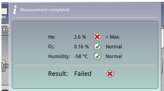
Measuring results are automatically compared with the defined limit values and an OK symbol is displayed if they pass.
