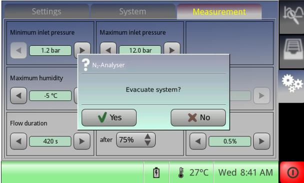
The screenshot shows the 'Measurement' menu with a confirmation dialog box for 'Evacuate system?'. The dialog box has 'Yes' and 'No' buttons. The background menu shows settings for Minimum inlet pressure (1.2 bar), Maximum inlet pressure (12.0 bar), Maximum humidity (-5 °C), and Flow duration (420 s).
