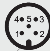
Circular connector M12 x 1, 5-pin
