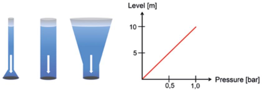
A static liquid generates, through its specific density and the acting force of gravity, a corresponding weight force or hydrostatic pressure which increases proportionally with the filling height. Consequently, the hydrostatic pressure represents a direct measure of the fill level or degree of filling of a tank or vessel.
